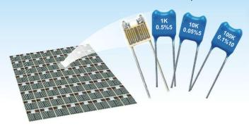
INTRON precision thin film resistors are made by vacuum depositing a controlled film of NiCr on high purity alumina substrate. The resistors are formed using high resolution photolithography. The values are micro trimmed to the exact value with a tolerance of 0.05%. The TCR and tolerance is obtained by process capability and does not rely on a selection process. Resistor sets matched to precise tolerance and TCR can be given.
